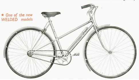
FRAME. Sizes 20". 21" or 22". Exclusive "C.B." design as illustrated with twin fine-taper struts to rear "triangle." Rigidity absolutely equal to gent's frame. Welded construction. Weight, approx. \$\frac{1}{2}\$ lb. (340 grammes) lighter than brazed frame. Built with a special alloy steel tubing (Accles & Pollock "S.A.Q." or Reynolds "531") which increases resistance to fatigue at, or near the joints. Taper butted seat
