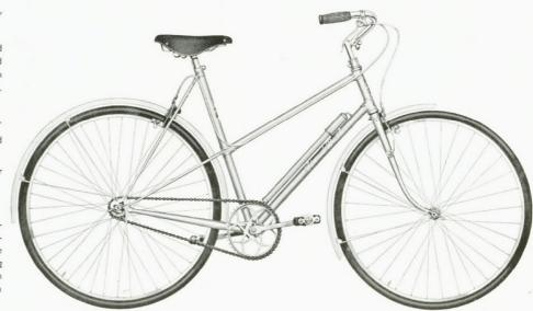
All frames receive anti-corrosive treatment prior to enamelling
