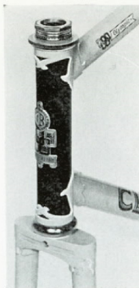
↑ HEAD ASSEMBLY showing lug cut-out and solid crown
