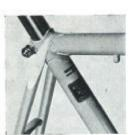
Constructed throughout from '531' doublebutted tubing and Continental Nervex 72° parallel lugs. Neatly finished seat cluster, Agrati ends and round-oval-round chain stays give a solid back, balanced by a low bottom bracket. Finely tapered oval blades are set into a sturdy fork crown.
