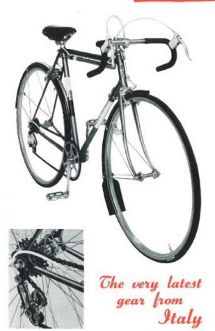
A road machine of proven design, built with Reynolds '531' tubing, which will withstand the rigours of club riding and racing, but give gentle handling in town traffic.
