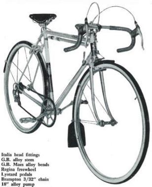
L15N saddle, chrome plated frame, perforated flap Williams C34 chainset with 6½" fluted cranks Bluencis Classique black guards with chrome strip Steel 27" H.P. rims on British Hub S.F. hubs Dunlop 27" Sprite amber walled tyres and tubes
