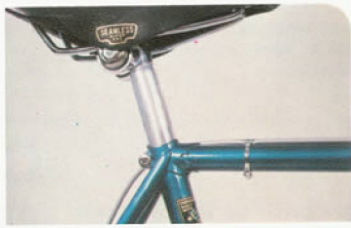
Sound frames based on top quality tubing some with Reynolds 531 butted
