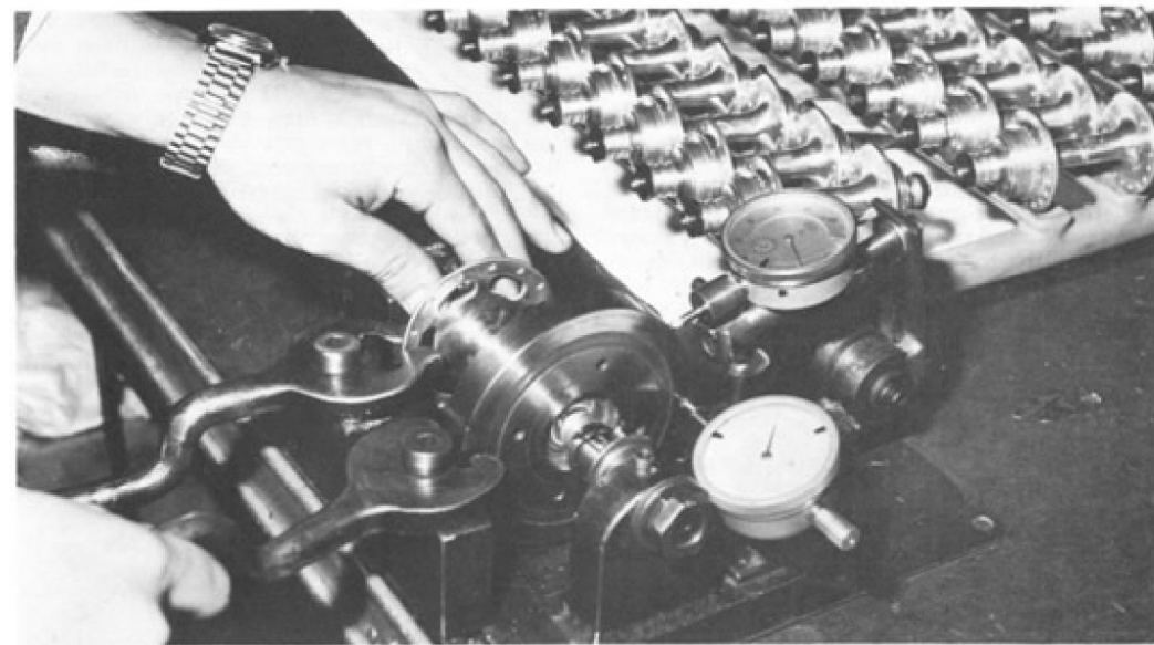
Inspecting the alignment of the flanges and the freewheel threads on a large flange hub.
