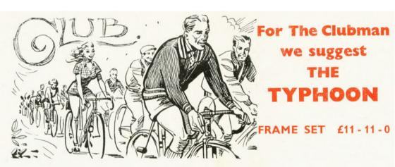
This light and lively mount is constructed with Continental Lugs cut to an attractive design, brazed into Reynolds best "531" or A. & P. "Kromo" butted tubing. Oval to round Fork Blades, 23" rake, frame angles 73° head and 71° seat, and with Continental-type head fittings
