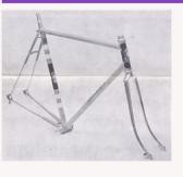
Fully sloping Prugnat fork crown of integral design with reinforcements concealed within the oval blades.
