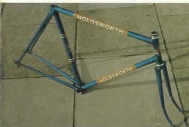
ROAD Angles 73" parallel. Short rake forks and rear triangle. Clearance for sprints and tubulars. Campagnolo road ends. No mudguard eyes. Brazed on gear stop and guide to chain stay only. Fitted with T.D.C. Italia or Milramo headset.
