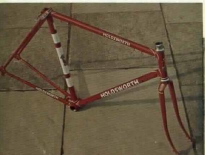
A high class frame built with slightly more clearance so that mudguards may be fitted if required. Still based on the Strada design but using a fork rake of 12" and a rear triangle of 17" with clearance for sprints with mudguards it still does not look "gappy" when stripped for racing. Campagnolo front and rear ends, choice of fully aloping integral or semi sloping fork crown, 8" fully wrapped over seat stays and 10½" bracket height. Brazed on fittings as required. Allen key seat fixing.
