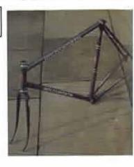
We are proud to offer these superb frames, hand built, using the famous Reynolds 531 tubing throughout and incorporating the Purposet Italian style lugs and fork crowns and featuring the Allen key seat bolt fitting.
